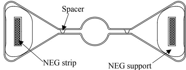
Figure 1: Concept of the vacuum chamber
