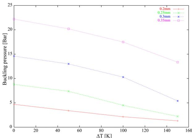
Figure 2: Evolution of buckling pressure as a function of the wall thickness and the temperature difference
