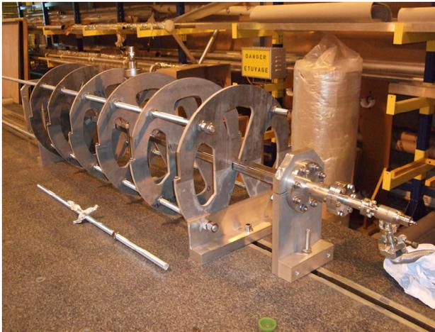
Figure 4: Test set-up of the vacuum chamber
