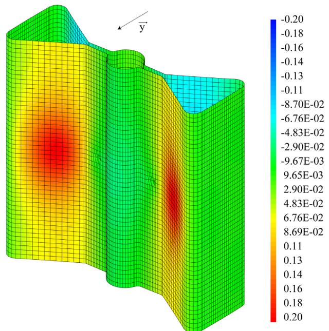
Figure 3: Typical buckling mode and related displacement in the  $y$  direction
