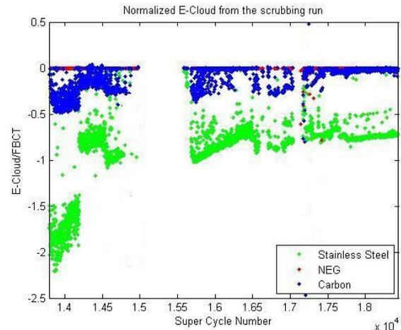
Figure 2: ECM signals from StSt, NEG and carbon (CKr4) liners during the SPS scrubbing run with (Super) cycle length of 43.2 s.
