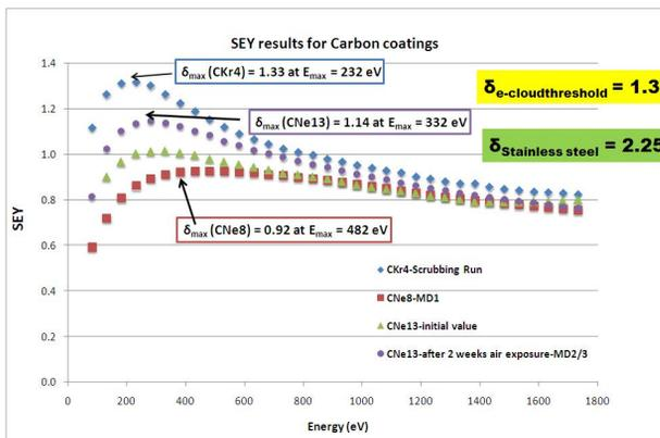
Figure 1: SEY of carbon coated liners before exposure to beam in the SPS as measured in the lab.
