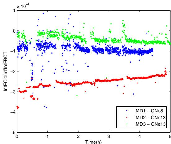
Figure 4: ECM signal (normalised to maximum beam intensity during the cycle) from amorphous carbon liners during the MDs with nominal LHC beam in the SPS.
