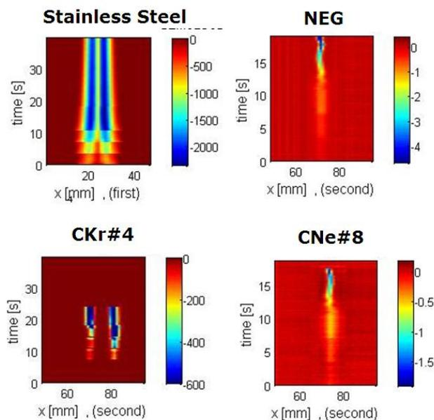
Figure 3: Electron cloud signal in ECMs with StSt, NEG and two carbon liners during scrubbing run (left) and acceleration (right) of nominal LHC beam in the SPS.
