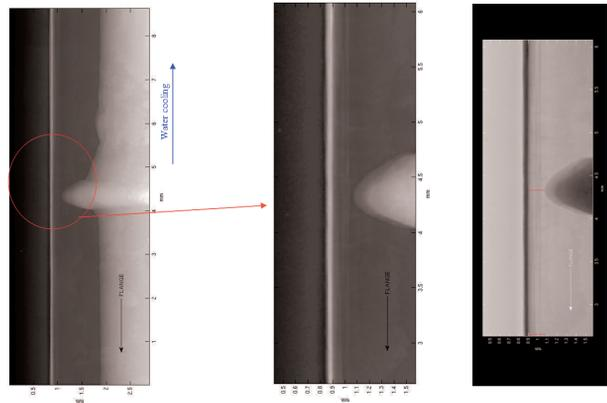
Figure 4: X-ray views of the damage created by high-energy photons on the cooling tubes of the crotch, as taken on ESRF ID6 beamline (courtesy J.C. Biasci, Front End Group ESRF).
