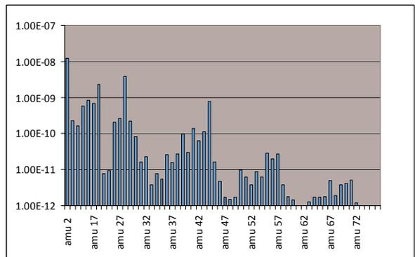
Figure 2: Residual gas analysis of a un-baked In-Vacuum undulator @ 200mA, first stored beam.
