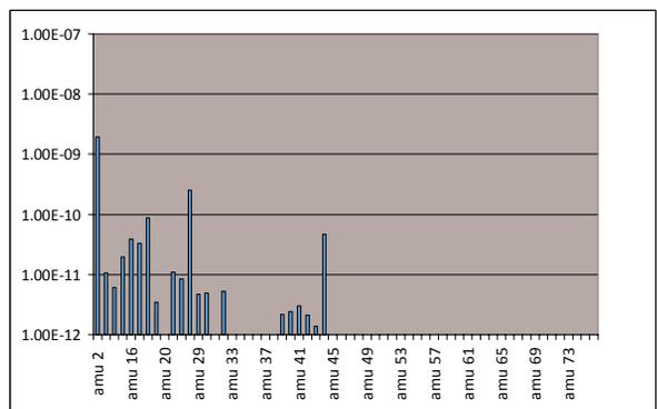
Figure 3: Residual gas analysis of a un-baked In-Vacuum undulator @ 200mA, 720 Ah accumulated beam.
