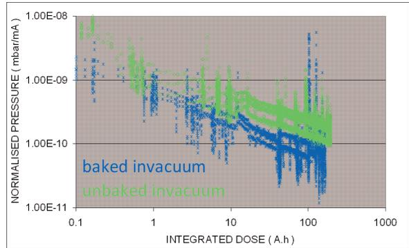
Figure 1: Vacuum conditioning behaviour of baked and un-baked 2-m long In-Vacuum undulators.
