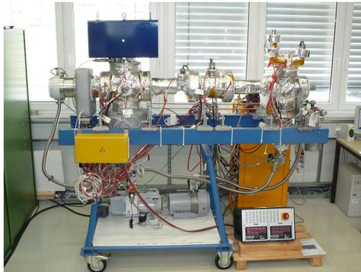
Figure 2: Picture of the experimental set up built to study the NEG ageing.
