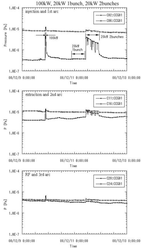
Figure 4: Variation of the vacuum pressure at each beam condition in Run 20.
