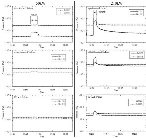
Figure 2: Variation of the pressure during the 50 kW and 210 kW beam operations.
