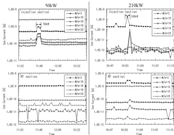
Figure 3: Variation of the outgassing components at injection and RF sections during the 50 kW and 210 kW beam operations.
