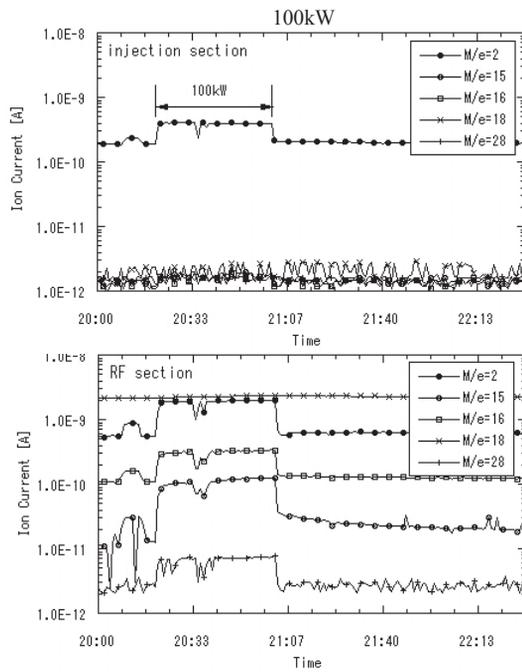
Figure 5: Variation of the outgassing components at injection and RF sections during 100 kW beam operation in Run 20.
