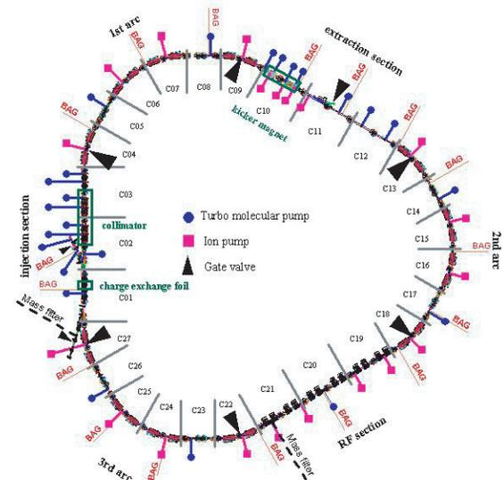
Figure 1: RCS vacuum system. RCS is conveniently divided into three straight and arc sections, which consist of 27 cells.
