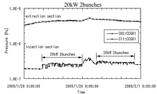
Figure 7: Pressure at injection and extraction section during 20 kW 2 beam bunches operation in Run21. Pressure increase between the beam operation is effect of a stop of the main magnet.
