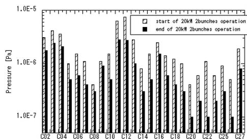
Figure 6: Comparison of the pressure between the start of the 20 kW 2 beam bunches operation and 10 hours later.
