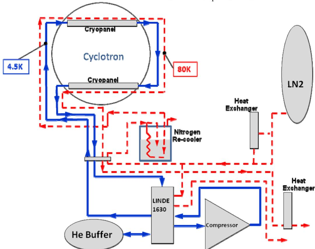
Figure 1: Cyclotron Cryogenic System Diagram.
