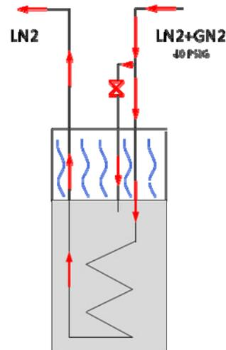
Figure 2: Nitrogen re-cooler.
