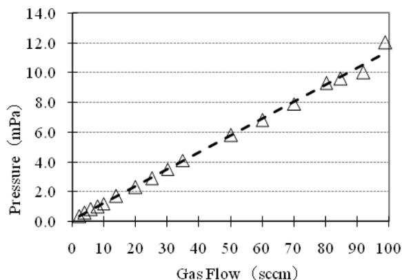
Figure 3: Test Cryopanel Pressure vs. Gas Flow.
