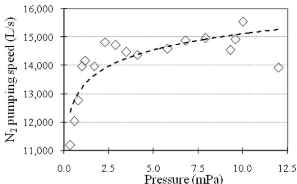
Figure 4: Test Cryopanel Pumping Speed vs. Pressure.
