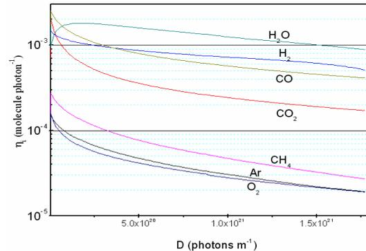
Figure 4: Result of the first PSD test for the chamber.
