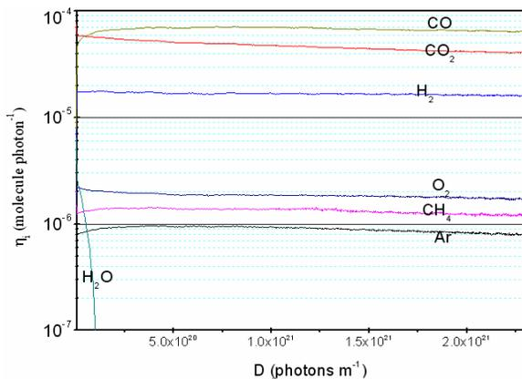
Figure 7: Final result of PSD test for TiN coated vacuum chamber after baking.
