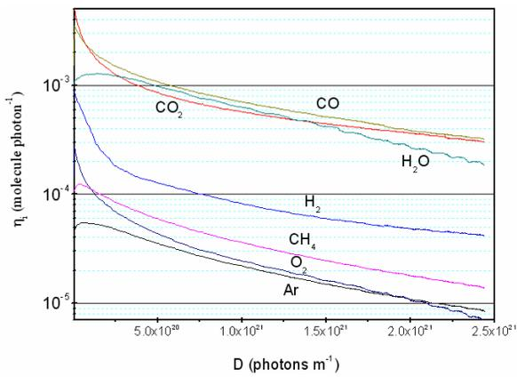
Figure 6: The first PSD test result for TiN coated vacuum chamber before baking.
