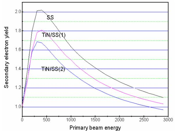
Figure 8: SEY results of stainless steel and TiN coated stainless steel samples under different condition.
