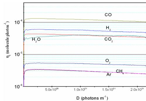
Figure 5: Final PSD test result for the chamber after baking.
