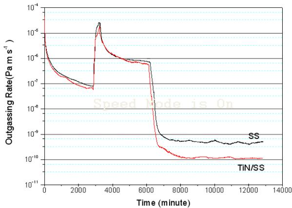
Figure 3: Compare of the outgassing rate for SS chamber and TiN coated SS chamber.
