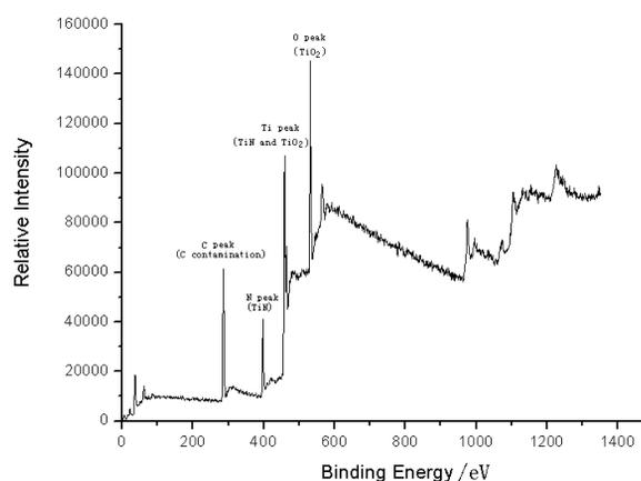
Figure 2: XPS survey spectra of the SS sample.
