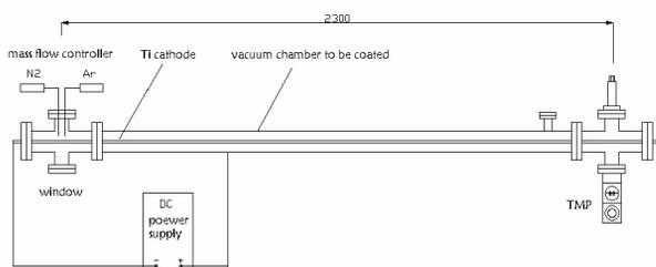
Figure 1: Schematic diagram of DC sputtering setup.
