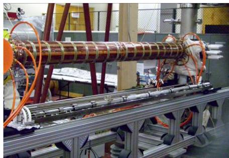
Figure 3: EBIS drift tube structure (below) and central vacuum chamber (above) where it will be inserted.
