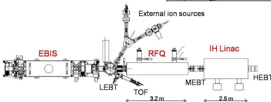
Figure 1: Layout of the EBIS-based heavy ion preinjector.
