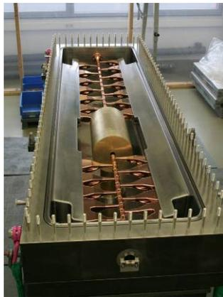
Figure 5: IH linac during initial rf testing.
