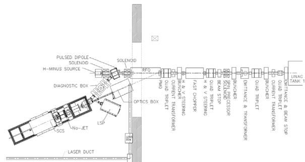
Figure 1: Layout of LEBT and MEBT before reconfiguration.
