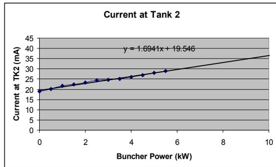
Figure 4: Linac output current as function of buncher power.
