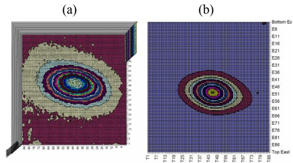
Figure 5: Beam foot print at the BLIP target (a) before and (b) after reconfiguration of LEBT/MEBT showing the same number of contours.
