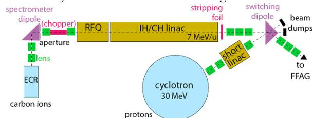
Figure 1: Schematic drawing of the beam injection into FFAG in the *PAMELA* project.
