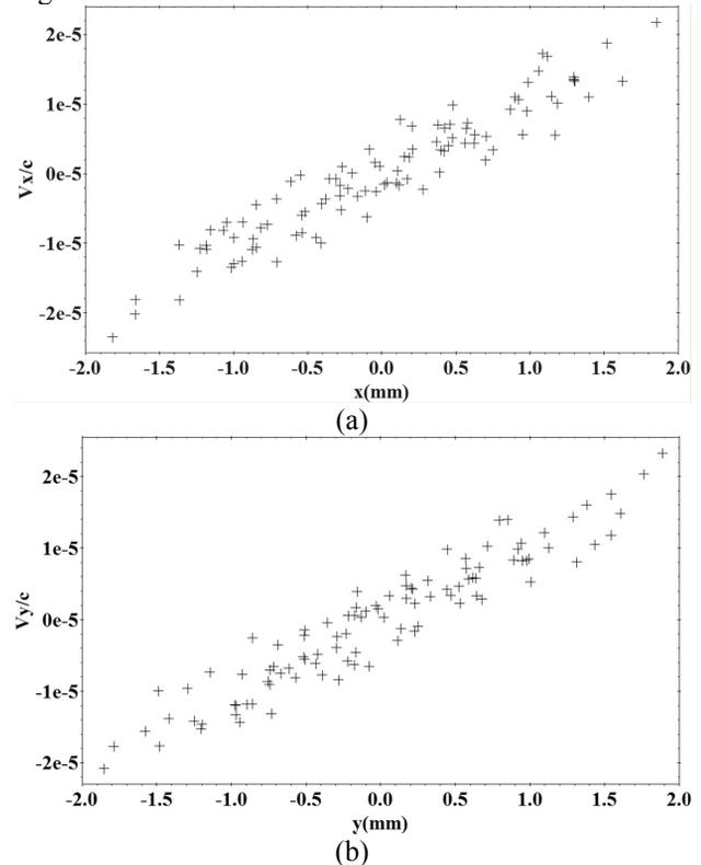
Figure 2: Initial (a) horizontal and (b) vertical phase space distributions of 100 sample particles starting from ion source.
