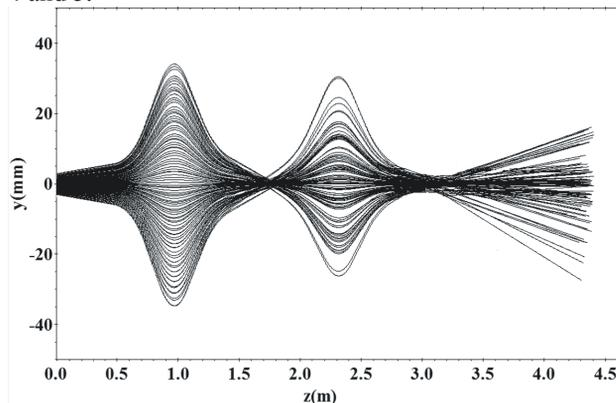
Figure 4: The trajectory of 100 particles in the vertical plane between the cyclotron and the FFAG ring, as obtained by GPT package. Two waists in the middle and at the end of the longitudinal direction correspond to the place where a buncher may locate and the entrance of the FFAG ring.
