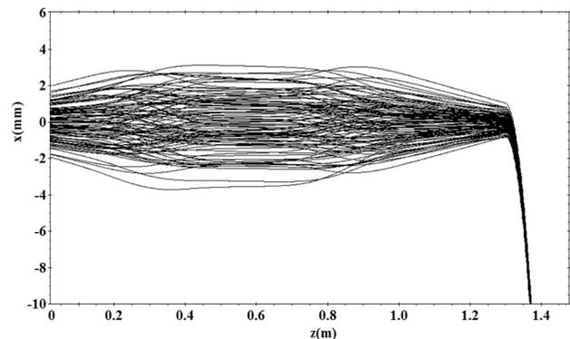
Figure 3: Two solenoids each 0.25 m long are positioned at 0.30 and 0.85 m from the ion source. The first solenoid runs the particles parallel and the second one focuses them. Each solenoid consists of 50000 Amp turns, with inner and outer radius of 0.05 and 0.10 m, respectively.
