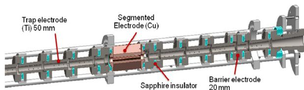
Figure 5: EBIT electrode system. The copper electrode in the centre of the Helmholtz arrangement is four fold segmented and allows direct view to the electron beam region.
