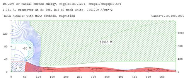
Figure 3: Electron gun simulation with the 6 mm cathode. The Wehnelt electrode is biased to -50 V for optimum beam formation.
