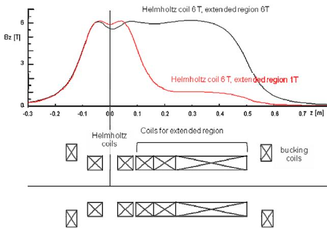
Figure 4: Magnetic field distribution the MSU EBIT.
