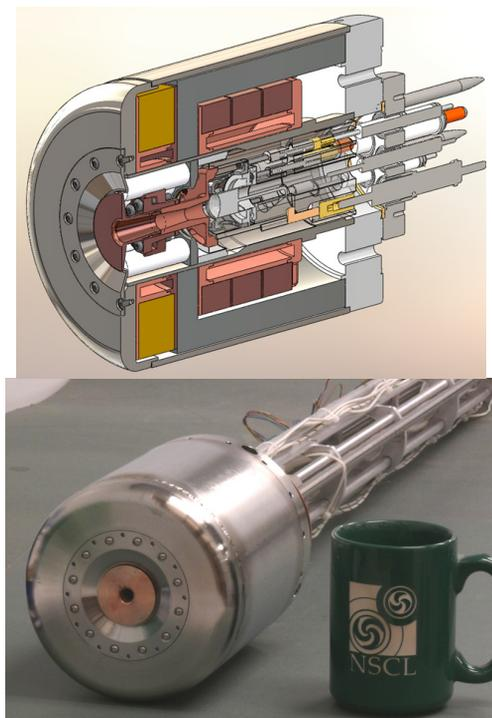
Figure 2: Electron gun of the MSU EBIT.
