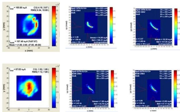
Figure 3:  $\text{Kr}^{13+}$  beam imaging using the current-scan technique (left) and transverse emittances (center and right). The top row corresponds to the ECR tune for maximum intensity. The bottom row corresponds to measurements done to a tune optimized for lower drain current but more homogenous distribution.
