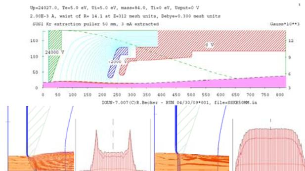
Figure 4: I-Gun calculations done for a Krypton beam. Top: potential profile for a 24kV beam and a puller gap of 50mm Bottom: (Left)  $\text{Kr}^{13+}$  and  $\text{Kr}^{17+}$  distributions for 2mA drain current. (Right)  $\text{Kr}^{13+}$  and  $\text{Kr}^{17+}$  distributions for 1mA drain current. Distributions are shown at the end position of the simulation.
