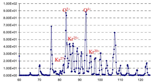
Figure 1: <sup>84</sup>Krypton distribution optimized on Kr<sup>25+</sup>
