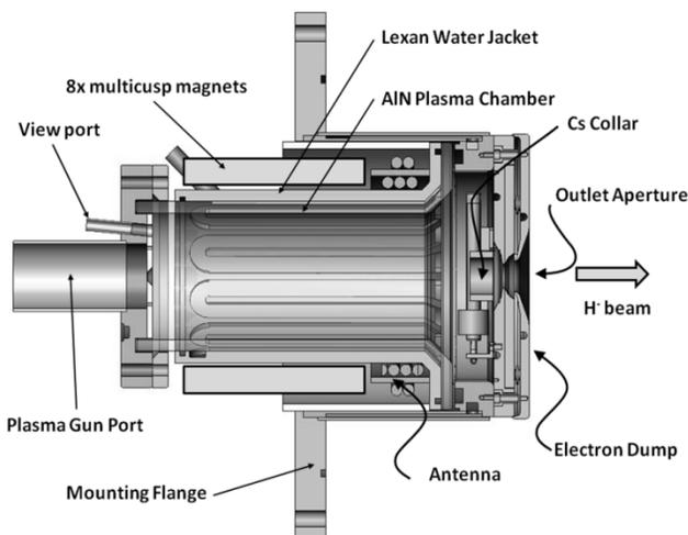
Figure 1: Schematic diagram of the SNS External Antenna Source (detailed view of collar shown in Fig. 2).
