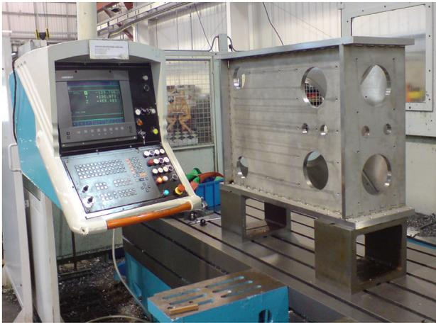
Figure 7: The vacuum vessel during manufacture.
