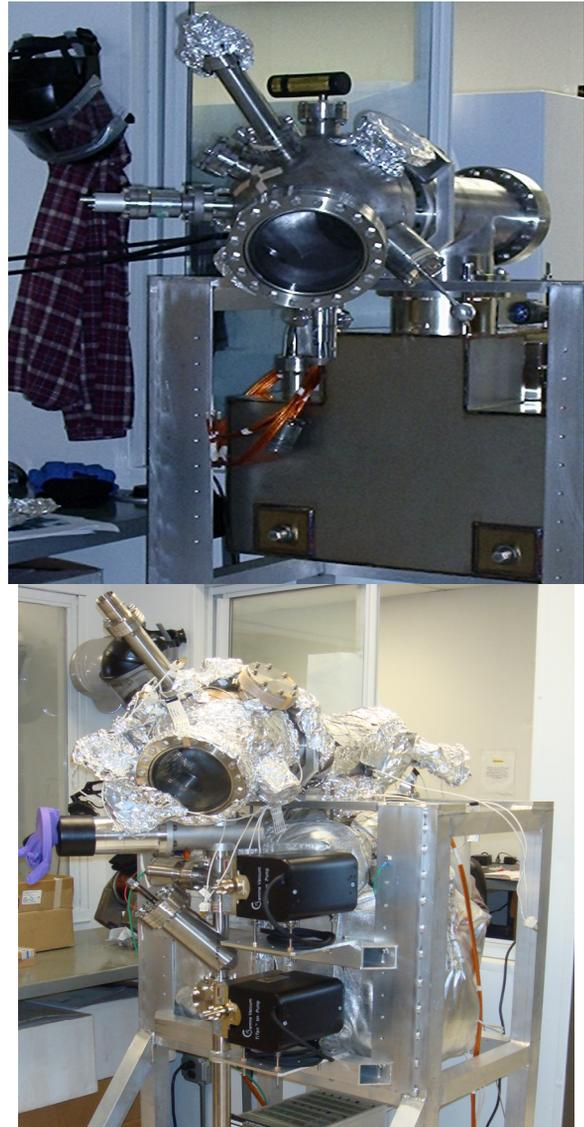
Figure 3: The preparation system on the top with attached TSP and on the bottom wrapped for baking with attached cathode transporter. The two ion pumps are part of the transporter.
