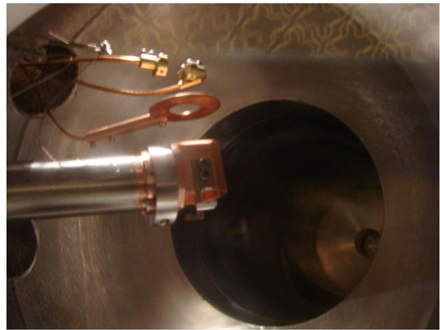
Figure 5: The cathode holder inside the preparation chamber is mounted on a heater stalk. The ring shaped anode is used to measure the quantum efficiency during preparation. Above the anode is the holder for the Cesium source. Not shown is a movable shield that can be inserted between the heater block and Cesium source to protect the source from radiated heat.
