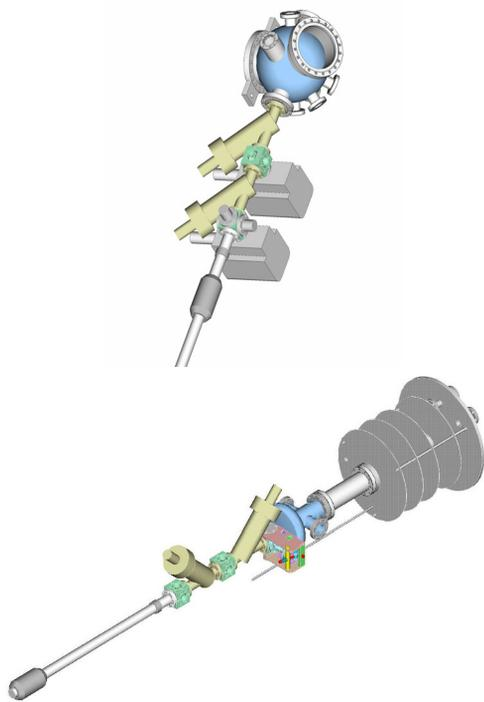
Figure 4: The transporter attached to the preparation chamber and to the gun assembly.
