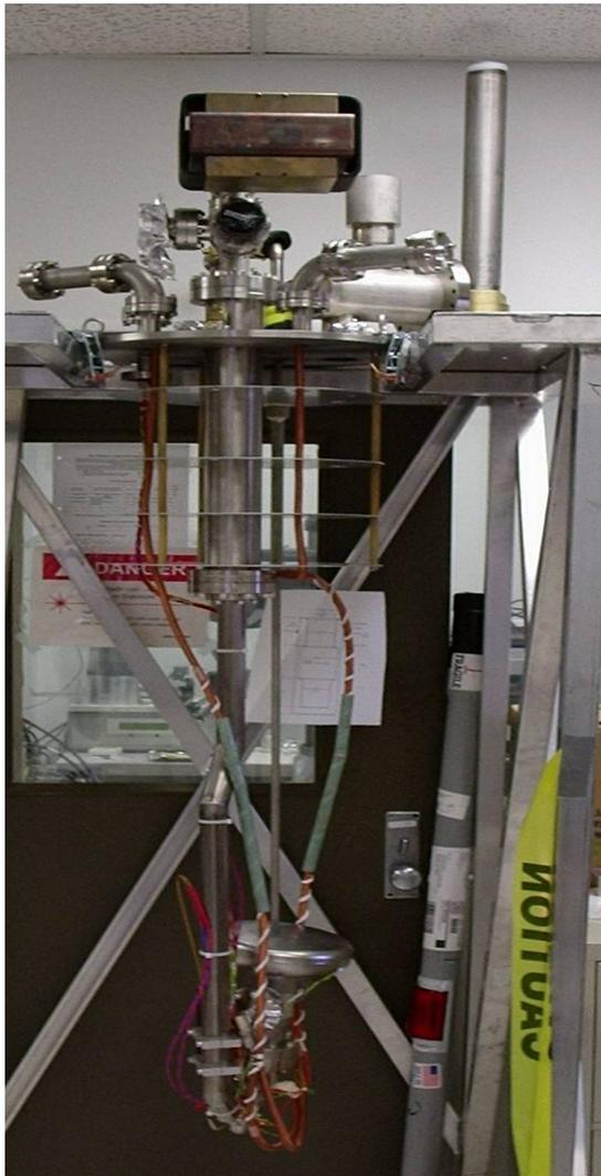
Figure 2: Gun assembly as used in the first cool down test. The gun is mounted upside down to prevent particulate from falling into the gun.
