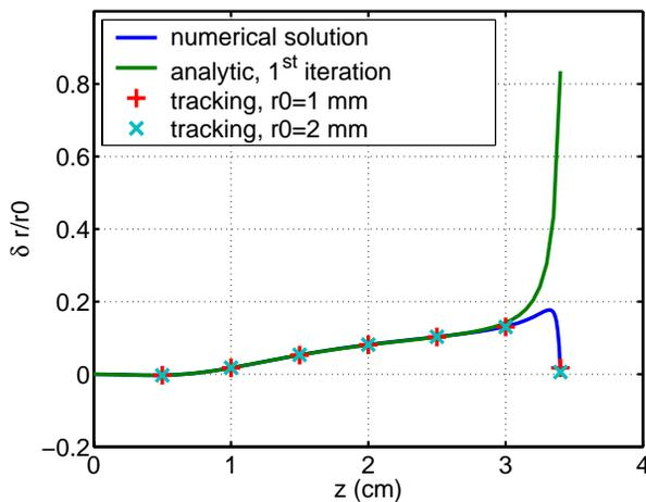
Figure 3: Normalized deviation of ion trajectories from the initial radius at the cathode as a function of the ionization coordinate. Tracking results for initial radii  $r_0 = 1$  mm and  $r_0 = 2$  mm practically coincide with each other, confirming the linearity of ion motion close to the gun axis.
