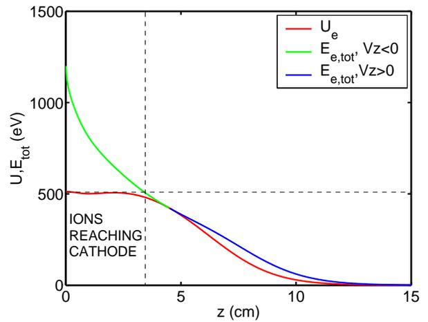
Figure 2: The effective potential energy (red) and the total effective energy (green and blue curves) of  $\text{H}_2^+$  ions in the BNL 1/2-cell SRF Gun. The green and blue curves, respectively, show the total energy of ions with the effective velocity  $\dot{x}_0$  pointing towards the cathode and away from the cathode.
