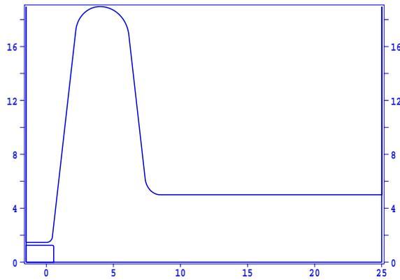
Figure 1: SuperFish model of the BNL 1/2-cell SRF gun. The horizontal axis corresponds to the gun axis.
