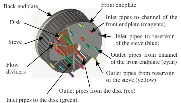
Figure 2: Cooling circuits for the 1-cell PWT.
