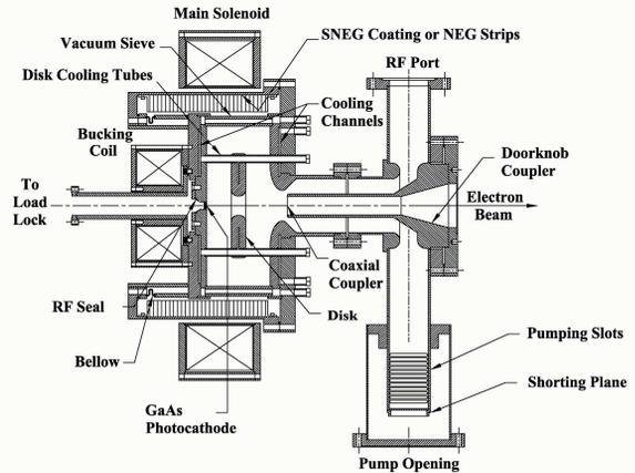
Figure 1: Schematics of a one-cell, CW L-Band PWT polarized electron gun.
