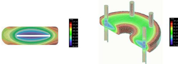
Figure 4: PWT disk temperature distribution (°F) from COSMOS/M 2D (left) and 3D (right) model.
