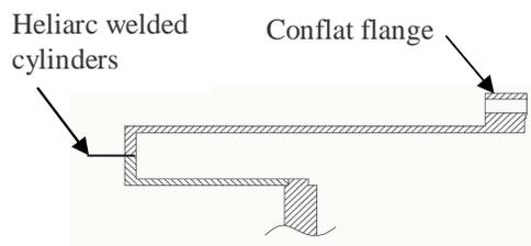
Figure 3: Heliarc welded design of the pressure vessel.
