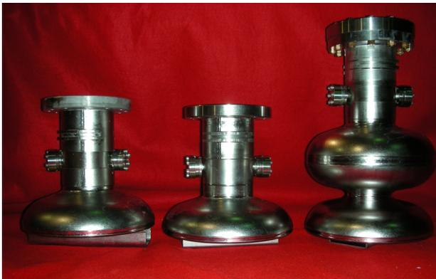
Figure 1: 1.3 GHz two half-cell and 1.6-cell SRF-gun cavities.
