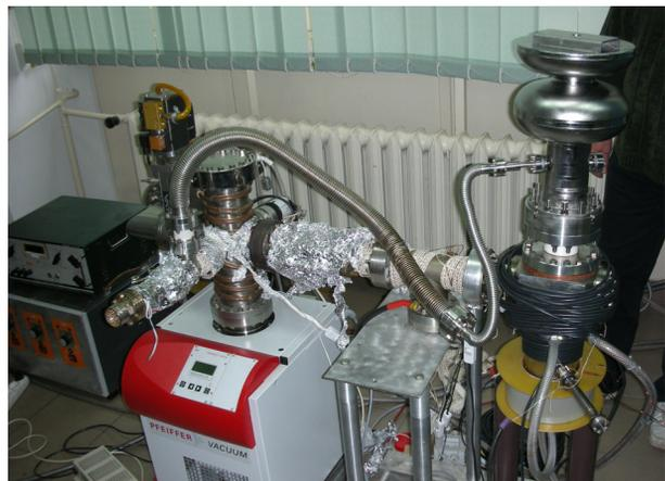
Figure 3: Setup for the plasma arc-deposition with the 1.6-cell cavity prepared for coating.
