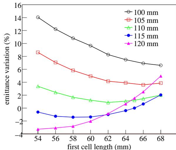
Figure 1: Normalised transverse emittance as a function of the first cell length for different second cell lengths.
