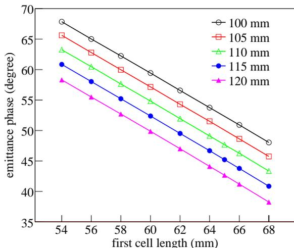
Figure 2: Beam optimum emission phase for highest beam energy as functions of cavity cell lengths.
