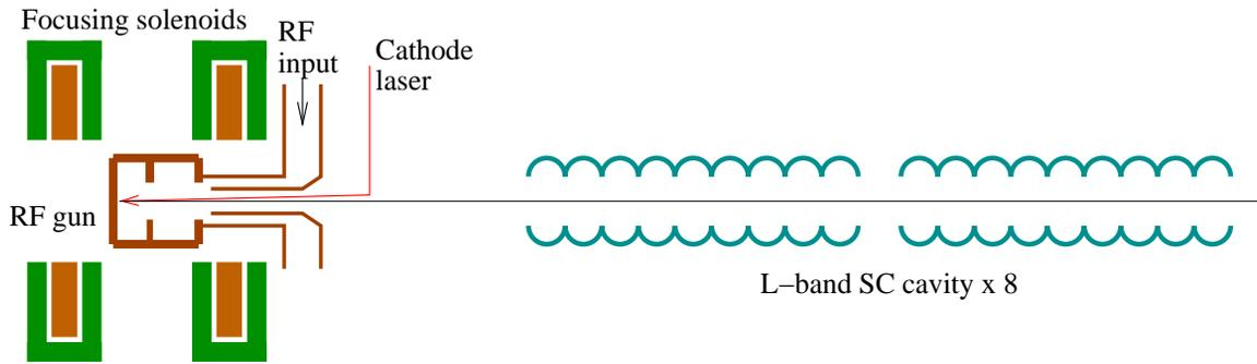
Figure 3: Layout of L-band normal conducting photoinjector.
