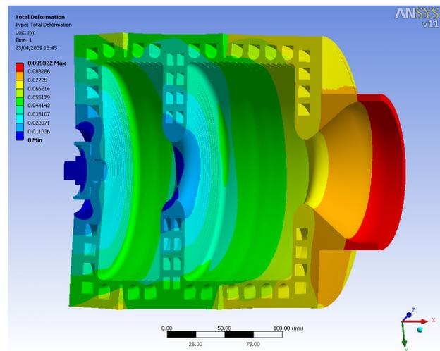
Figure 4: Cavity deformation by the stress distribution in Fig. 3. The deformation is magnified for visualisation.
