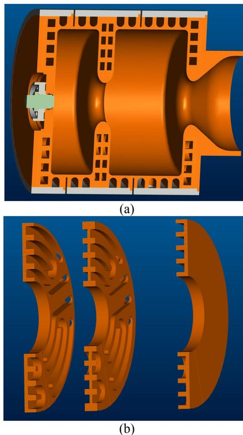
Figure 1: Gun cavity geometry and cooling-water channels. A cut of cavity geometry (a) and cooling water channels in the back plane and irises (b). Dark red colour presents the material is OFHC copper, pale green molybdenum and bright grey stainless steel.
