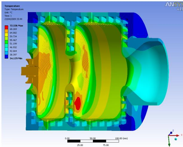
Figure 2: Temperature distribution over the cavity for 70 kW RF average power.
