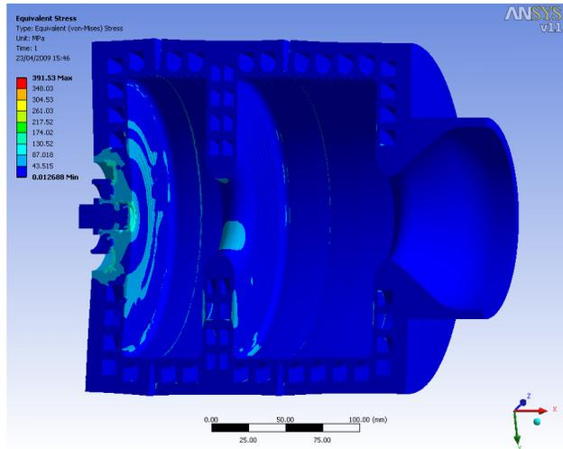
Figure 3: Stress distribution for the temperature distribution in Fig. 2. The deformation is magnified for visualisation.
