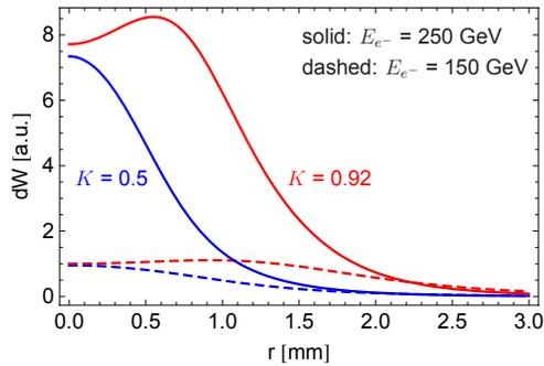
Figure 2: Undulator radiation at target surface for  $E_{e^-} = 250$  GeV (solid) and  $E_{e^-} = 150$  GeV (dashed) with  $d_{UT} = 500$  m,  $K = 0.92$  (red) and  $K = 0.5$  (blue) in the normalization  $dW(K = 0.92, E_{e^-} = 150 \text{ GeV}, \theta \rightarrow 0) \equiv 1$ .
