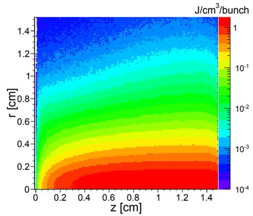
Figure 4: Energy density from a FLUKA simulation of the initial energy deposition into a 15 mm thick Ti-6%Al-4%V target by one bunch of the undulator radiation for  $K = 0.92$ ,  $\lambda_0 = 11.5$  mm and  $d_{UT} = 500$  m.
