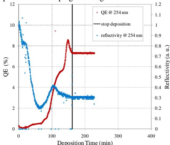
Figure 4: Reflectivity and QE at 254nm vs. deposition time for cathode 104.2.
