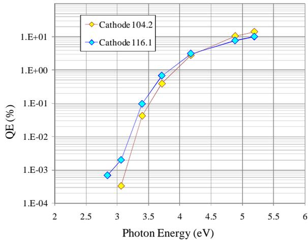
Figure 1: The final spectral responses of cathode 104.2 (10 nm Te) and 116.1 (5 nm Te).
