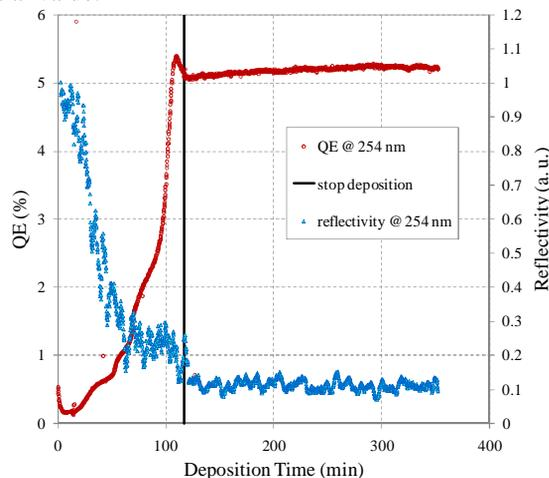
Figure 5: Reflectivity and QE at 254 nm vs. deposition time for cathode 116.1.
