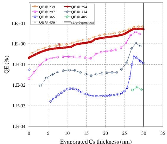
Figure 3: QE at different wavelengths vs. Cs thickness for cathode 116.1.
