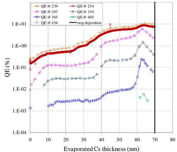
Figure 2: QE at different wavelengths vs. Cs thickness for cathode 104.2.
