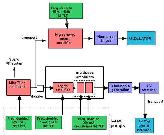
Figure 1: Conceptual drawing of the SPARC laser system.
