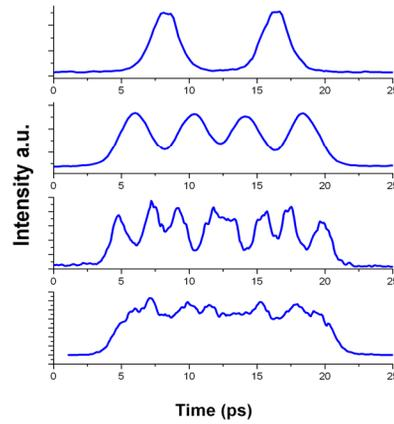
Figure 5: Step-by-step pulse shaping obtained with birefringent crystals.
