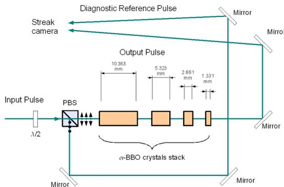
Figure 4: Schematic layout of the UV shaper based on the birefringent crystals.
