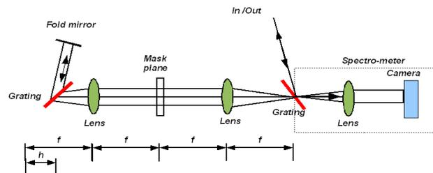
Figure 2: Schematic layout of the UV stretcher.
