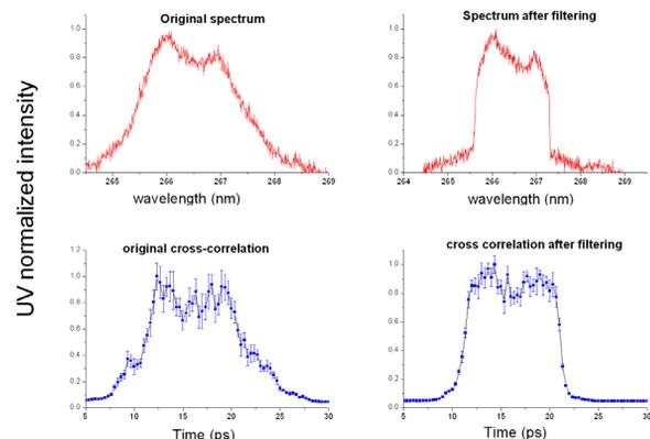
Figure 3: Spectral and time UV distribution obtained without and with the spectral filtering in the stretcher Fourier plane.
