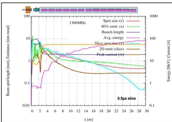
Figure 3. APEX injector beam parameters. (Case 2)
