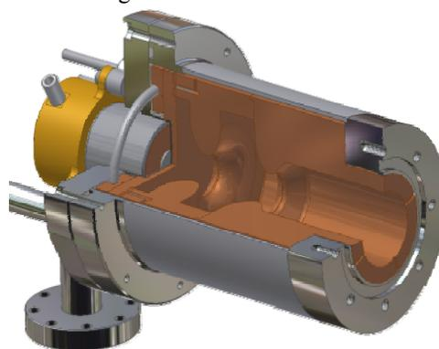
Figure 1: Schematic design of the 1.5-cell 2<sup>nd</sup> generation Dutch RF-photogun.
