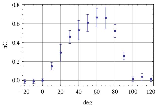
Figure 2: Photo-emitted charge vs. launch phase, with a laser-pulse energy of  $5.4 \mu\text{J}$ . The location of the zero phase is approximate. Error bar half-height is one standard deviation.
