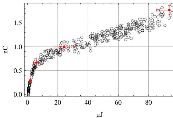
Figure 3: Photo-emitted charge vs. laser-pulse energy.
