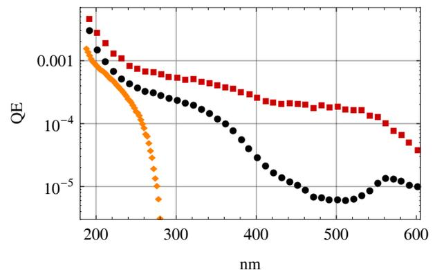
Figure 1: Test stand QE measurements. Circles and squares are data for the dispenser cathode, the former corresponding to zero cathode heating and the latter to 1.5 W in the resistive heating element embedded in the cathode. For reference, QE measurements on a copper cathode for the LCLS are shown as diamonds.
