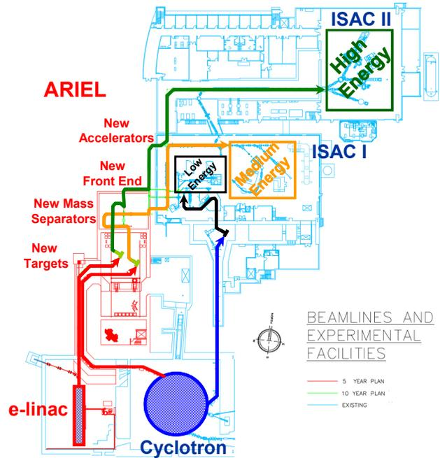
Figure 1: ARIEL project (red highlights) on the TRIUMF site. The present TRIUMF 500MeV cyclotron is driver to one of two production targets in ISAC. A new electron linac will add a complimentary driver to a new target facility while a second beamline from the cyclotron adds a drive beam to a third target allowing simultaneous RIB delivery to the three main experimental areas in ISAC-I and II.
