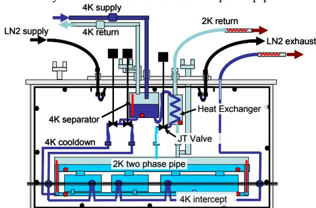
Fig. 5: Cryomodule cryogenic circuit showing cold mass, 4K phase separator, JT valve and heat exchanger.
