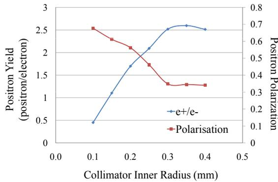
Figure 2: Positron yield and polarization as functions of collimator aperture.
