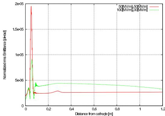
Figure 5: GPT simulation of the rms emittance along the linac from the cathode surface to the end of solenoid. The RF gun locates from 0 to 0.12[m] and solenoid from 0.2 to 0.4[m]. The simulation conditions are ; Number of particles 2000, total electron charge 500[pC], laser radius 1[mm], laser pulse length 10[pC], the peak solenoid magnetic field 0.3[T].
