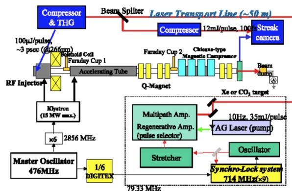
Figure 1: System of 18MeV Photocathode Electron Linac at the University of Tokyo.
