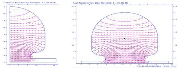
Figure 6: Pre-designed side-couple  $\pi/2$ -mode S-band RF gun by SUPERFISH.
