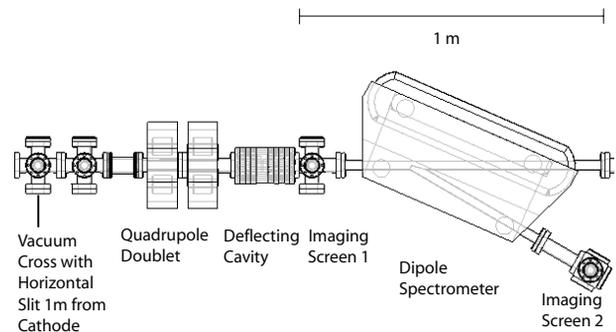
Figure 1: Experimental apparatus used to measure the longitudinal profile and longitudinal phase space of the photoinjector blowout beam.
