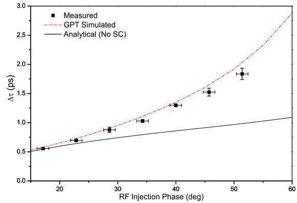
Figure 3: Measured time separation of centroids as a function of RF photogun injection phase.
