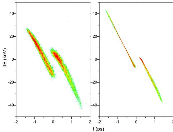
Figure 4: Measured and simulated longitudinal phase space of the double beam. The beams' respective charges were 5.7 and 5.3 pC, RF injection phase was 25 degrees, and the transverse spot size on the cathode was  $\sigma_x = 500 \mu\text{m}$  rms
