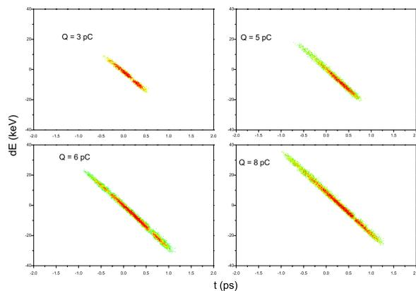
Figure 5: Four LPS's taken for different charges. As the charge is increased the variation in the beam chirp reduces due to the effects of the space charge induced expansion.
