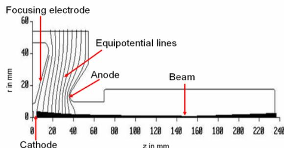
Figure 2: Beam transport inside the gun for the EIMAC Y-845 cathode and for a current of 0.2 A.
