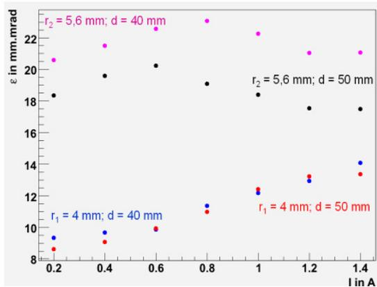
Figure 4: Emittance as a function of the current and the distance d between cathode and anode. Results are shown for the Y-845 cathode with  $r_1 = 4$  mm and YU-171 with  $r_2 = 5.6$  mm
