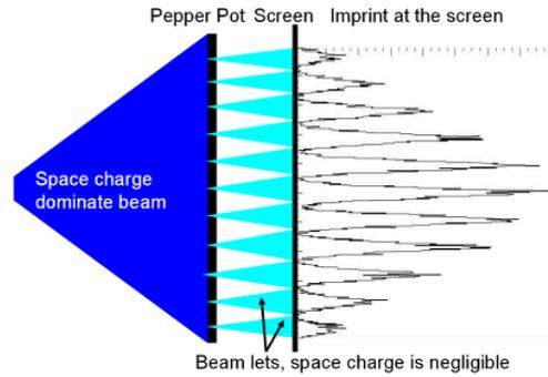
Figure 5: Principle of emittance measurement with a “Pepper Pot” device
