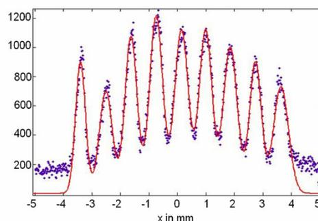
Figure 8: Emittance measurement for a current of 270 mA. The top plot shows the image from the “Pepper Pot” device, at the bottom the horizontal projection of the marked row is shown.
