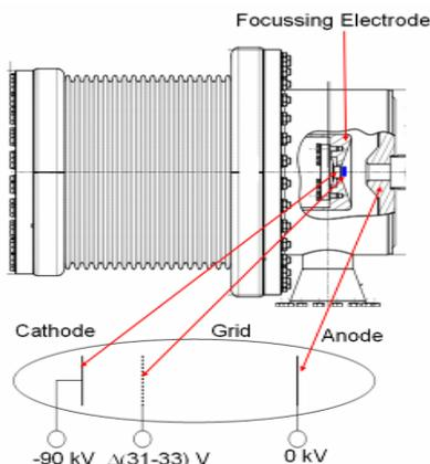
Figure 1: Design of the new electron source for ANKA. The grid voltage is given for multi bunch operation (compare with table 1)
