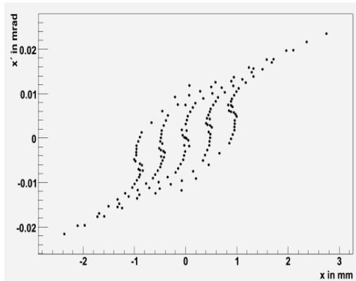
Figure 3: Expected phase space distribution after point reflection, calculated with the EGUN code at a distance of 235 mm from the cathode for a current of 0.2A.
