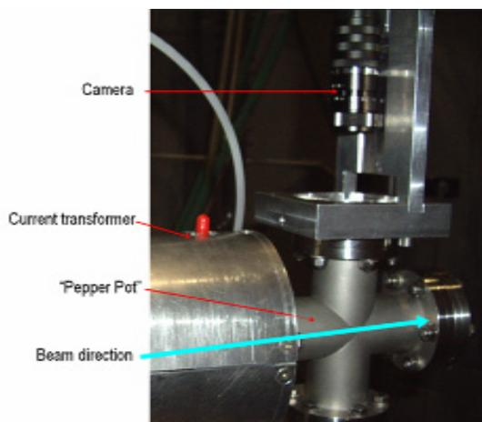
Figure 7: Experimental setup for the emittance measurement.
