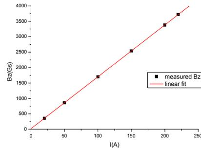
Figure 7: Peak magnetic field versus excitation current.
