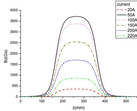
Figure 6: Measured axial magnetic field of the emittance compensation solenoid for different excitation current.
