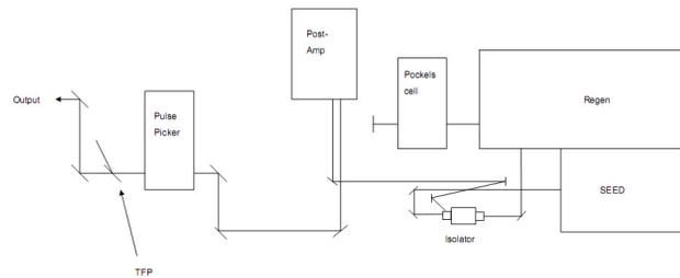
Figure 4: Principal optical setup of IC-10000 ps ND:VAN REG AMP.
