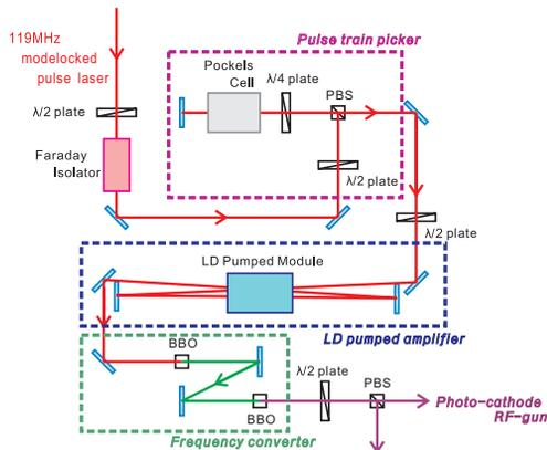
Figure 6: Multi-Pulse Laser System.
