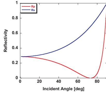
Figure 5: Reflectivity of Cs-Te as a function of Incident Angle.
