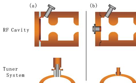
Figure 1: (a)Former Photo-cathode RF-gun system (b)Improved Photo-cathode RF-gun system.
