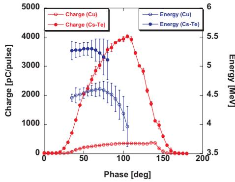
Figure 3: Charge and Energy measurement as a function of laser injection RF phase.
