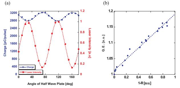
Figure 4: (a) Charge and Laser Intensity as a function of Angle of Half Wave Plate (b)  $Q.E. \propto (1 - R)$ .
