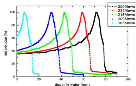
Figure 16: The Bragg-peaks in water for 5 energy-values.
