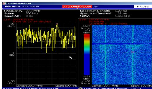
(a) C-beam Schottky signal with e-cooling.
