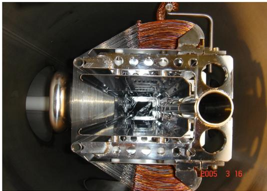
Figure 7: The electric-static septum of CSR.
