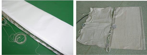
Figure 4: The UHV back-out jacket for dipole chamber.
