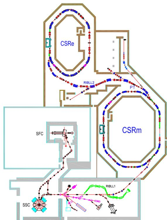
Figure 1: Overall layout of HIRFL-CSR.
