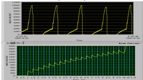
(a) C-beam current during STI + e-cooling and ramping.
