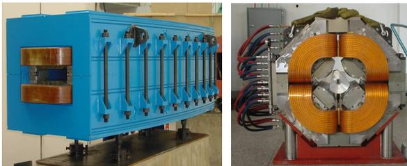
a) Dipole of CSRm.      b) Quadrupole of CSRm.
