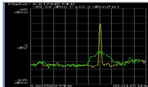
Figure11: Schottky signal of cooled C-beam in CSRe.
