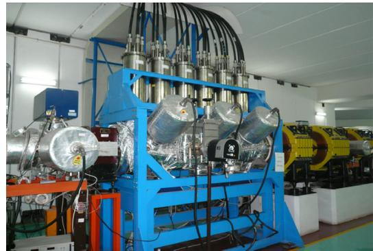
Figure 8: The fast-pulse kicker of CSRm.
