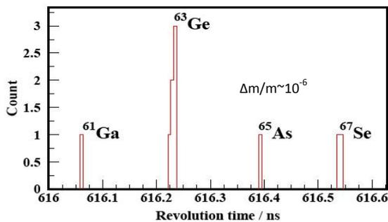
Figure 13: The RIBs mass-measurement result in CSRe.
