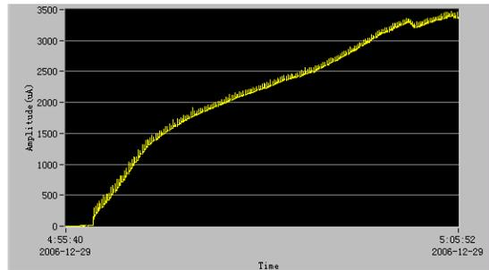
(b) C-beam accumulation with STI + e-cooling.
