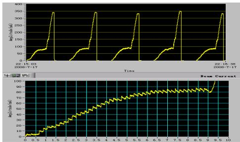
(c) Kr-beam current during MMI + e-cooling and ramping.
