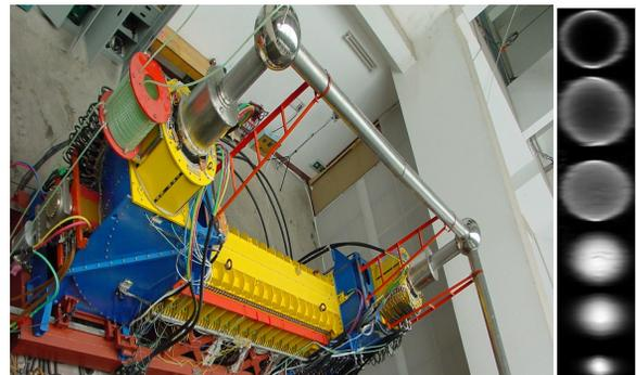
Figure 5: The e-cooler of CSRm and the hollow e-beam.
