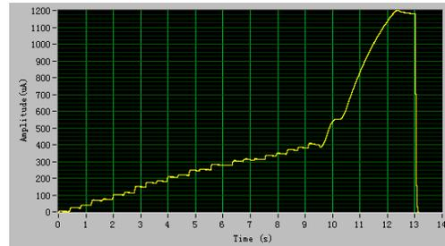
(b) Ar-beam current during MMI + e-cooling and ramping.
