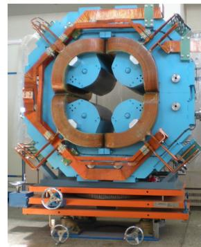
Figure 9: The prototype quadrupole magnet
