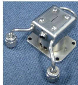
Figure 3: H<sup>-</sup> Pinning source body tested at ISIS.
