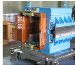
Figure13: The prototype injection bump magnet.
