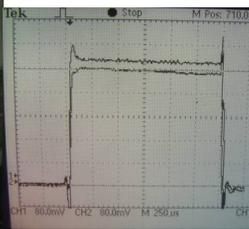
Figure 6: Measured input and output beam current.
