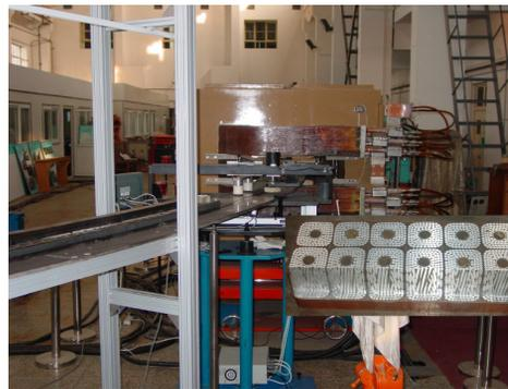
Figure 8: The prototype dipole magnet of stranded coil and the measurement system
