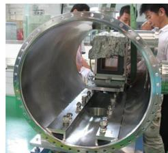
Figure 15: The prototype extraction kicker magnet.
