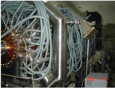
Figure 5: 352MHz RFQ for an ADS basic study program has been built at IHEP, Beijing.
