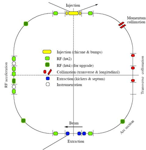
Figure 2: Functional layout of the CSNS synchrotron with four straights sections mainly used for beam injection, transverse and longitudinal collimation, acceleration, and extraction
