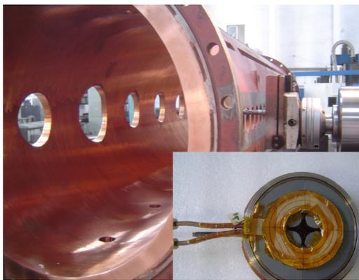
Figure7: Prototype of the DTL tank and drift tube
