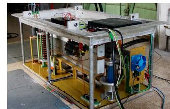
Figure16: The prototype pulse power supply for the extraction kicker magnet.
