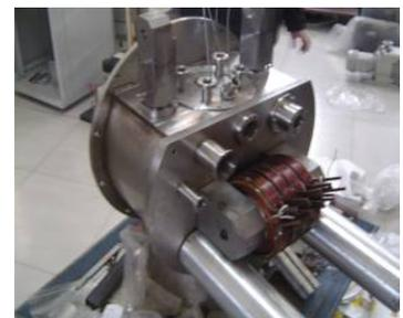
Figure 4: An Penning source test stand is setting up at IHEP.
