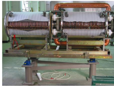
Figure 12: The prototype of the ferrite loaded RF cavity.
