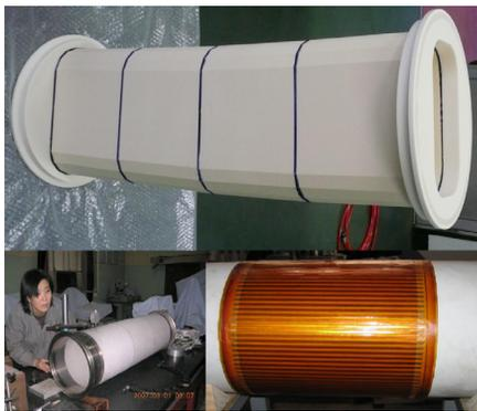
Figure 11: The short prototype of the dipole ceramic chamber (upper) and two full-size quadrupole ceramic chambers (lower).
