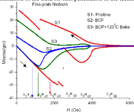
Figure 4: M vs H to obtain  $H_p$  in fine grain samples.
