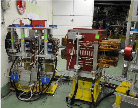
Figure 2: Dipole magnet (red) and dipole vacuum chamber installed in TL2 at CERN
