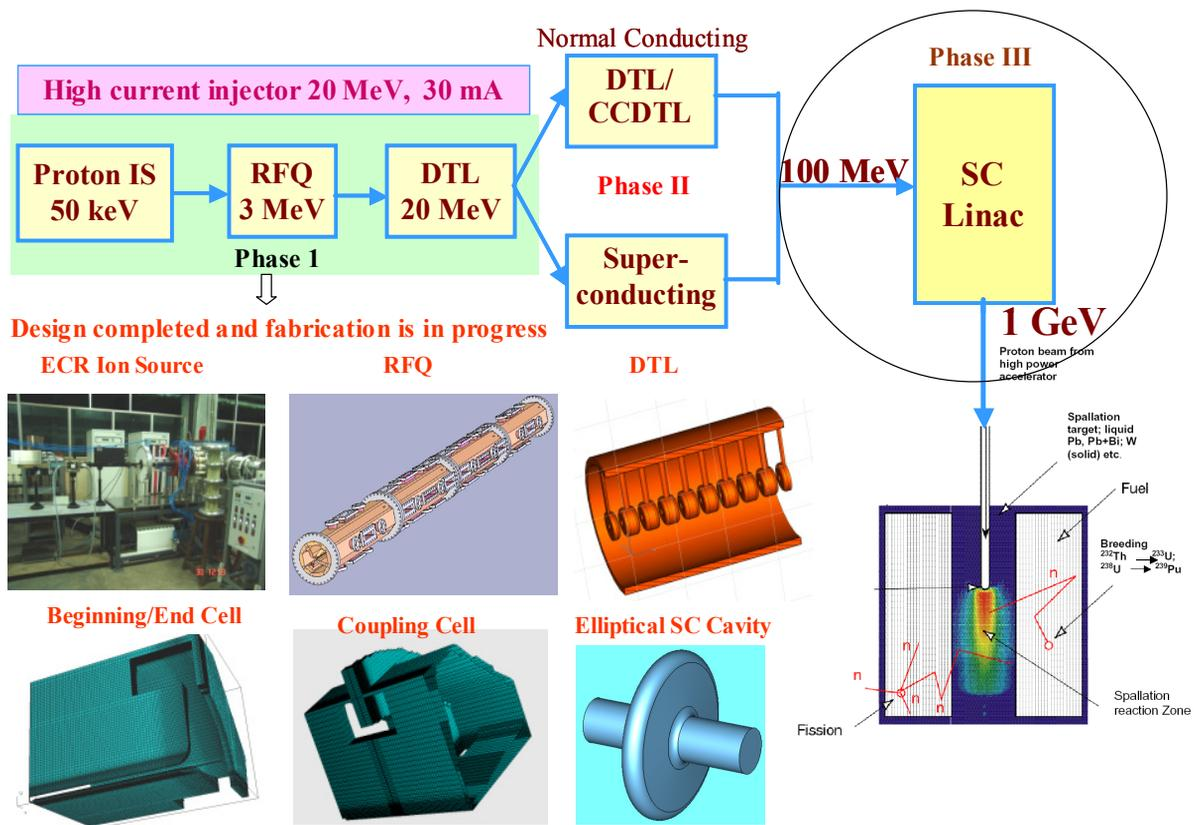
Figure 6: Scheme of high intensity proton accelerator started by BARC for ADS linked R&D. Work on phase I is on.
