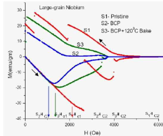
Figure 5: M vs H to obtain  $H_p$  in large grain samples.
