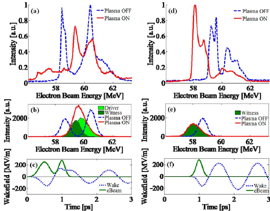
Figure 1: Experimental and simulated energy spectra after the 6 mm-long capillary discharge at  $1 \times 10^{16} \text{ cm}^{-3}$  plasma density for the double-bunch beam (left column), and for the witness bunch only (right column): (a), (d): experimental energy profiles; (b), (e): simulated energy profiles; (c), (f): simulated plasma wakefield and position of the bunches inside the wake.
