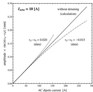
Figure 4: Amplitude of the driven beam (multiplied by a factor  $\sin[\pi(\nu_d - \nu_0)]$ ) vs. amplitude of the AC dipole's current. The detuning effect either suppress or enhance the beam's amplitude. The deviation of the beam's amplitude from the linear growth allows to determine the detuning effect.
