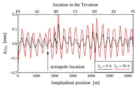
Figure 2: Central orbit distortions due to sextupole fields when the current of the controlled sextupole magnet is 0 A (nominal) and 30 A. When the current is increased to 30 A, the effect grows as expected ( $\sim 80 \mu\text{m}$ ) and shows a cusp structure, indicating location of the sextupole magnet.
