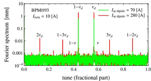
Figure 6: Fourier spectra of turn-by-turn positions of the AC dipole's excitations. The peaks at  $2\nu_d$ ,  $1 - 2\nu_d$ ,  $3\nu_d$ , and  $1 - 3\nu_d$ , corresponding to the modes driven by the sextupole and octupole fields, appear only for the larger excitation, indicating these modes depend on the oscillation amplitude of the AC dipole's excitation.
