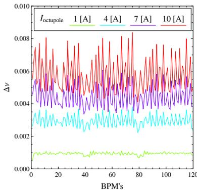
Figure 5: Tune shifts measured with all the BPMs for different currents of the controlled octupole magnets. The driving tune and the maximum amplitude of the AC dipole are fixed to  $\nu_d - \nu_0 = -0.015$  and 280 A, producing 5 mm oscillation amplitude in the arc.
