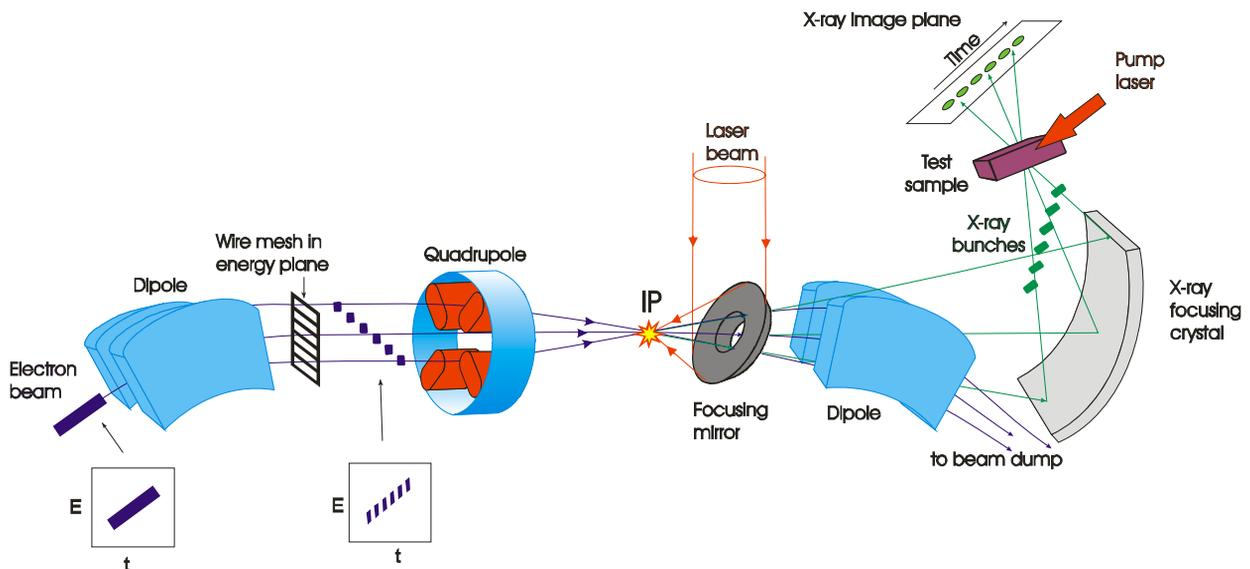
Figure 6: Simplified schematic of our proposed x-ray stroboscope.
