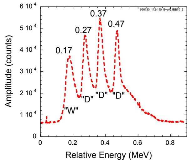
Figure 5: Projection at the energy spectrometer illustrates difference in energy change after passing through two dipoles for the last (W) and prior (D) bunches, when compared to Fig. 4.
