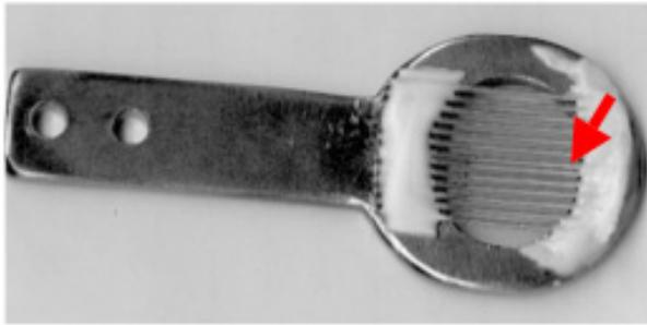
Figure 3: Picture of the wire mesh mask and frame. The wires are  $d=800$   $\mu\text{m}$  in diameter with a period of  $D=1650$   $\mu\text{m}$ . The red arrow indicated the two consecutive wires.
