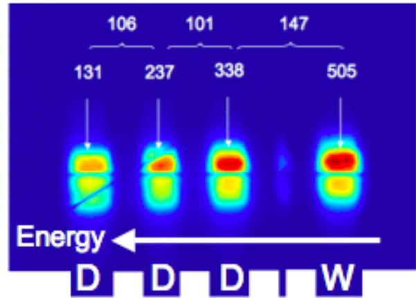
Figure 4: Shadow cast by the wire mesh captured 286 cm downstream from the mask, in the dogleg. Three DBs and one WB have been selected with the energy slit. The slit and the mask wires are schematically indicated by the white rectangles at the bottom of the image. The numbers indicate the bunch locations on the image, as well as their calculated separation (in pixels). The two lines across the image are caused by alignment wires on the screen.
