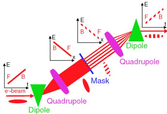
Figure 1: Simplified schematic of the mask principle. Only the dogleg section of the beam line is depicted (not to scale), and three quadrupole magnets are omitted. The side graphs represent the beam energy correlation with the beam front labeled by “F” and the back by “B.”
