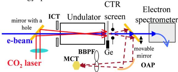
Figure 1: A schematic of the experiment. ICT is an integrating current transformer, BBPF - a broadband-pass filter, MCT - a Mercury Cadmium Telluride detector.
