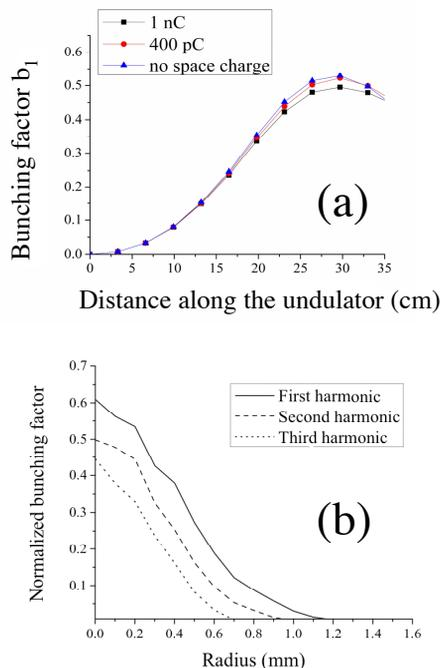
Figure 3: 3-D simulations. Dependence of the bunching factor  $b_1$  along the undulator for different beam charges (a) and normalized bunching factor for the first, second, and third harmonic of the microbunched beam at the exit of the undulator versus the electron beam radius (b).
