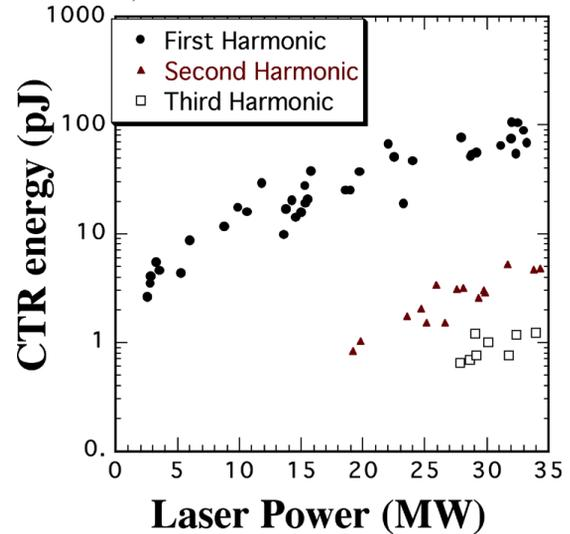
Figure 2: CTR energy for the first, second, and third harmonics as a function of CO<sub>2</sub> laser power for the 12.3 MeV beam.
