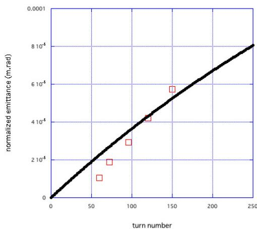
Figure 5: Emittance growth in the vertical direction as a function of turn numbers. Vertical axis in this figure shows a normalized emittance. Open squares show the experimental results and a solid line shows the theoretical estimation based on the ionization cooling model.
