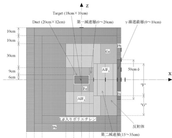
Figure 3: Schematic configuration of neutron moderator.
