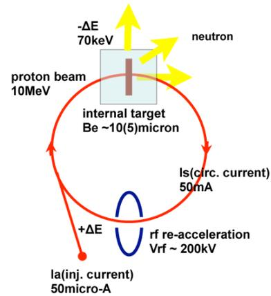
Figure 1: Schematic diagram of FFAG-ERIT.
