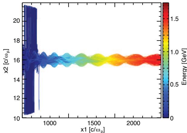
Figure 2: Projection of the trajectories of the self-injected particles in the LWFA for the 1.5 GeV configuration. Particles move from the left of the right, and are mostly injected off-axis. Color represents energy.
