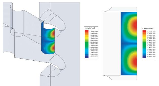
Figure 8: 14 MV/m electric field on inner rod for 5.9 MW, or 100 MV/m gradient.
