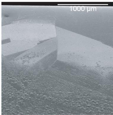
Figure 6: SEM micrograph showing detail of inner rod pulsed heating damage.
