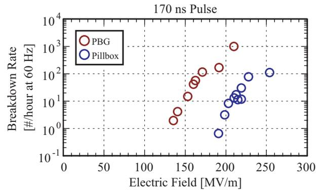
Figure 2: PBG and pillbox breakdown rate vs. maximum surface electric field.
