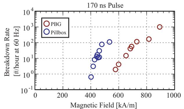
Figure 3: PBG and pillbox breakdown rate vs. maximum surface magnetic field.
