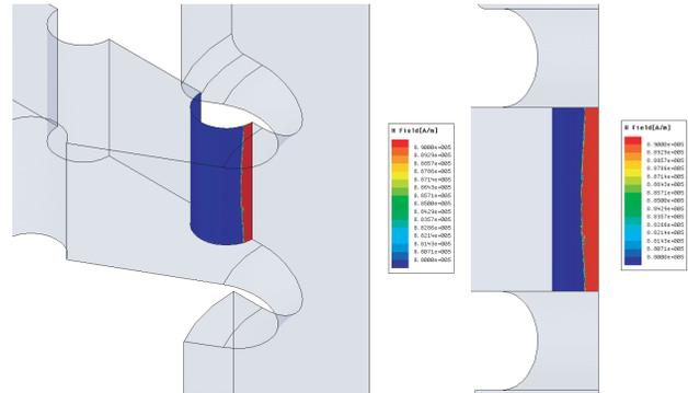
Figure 7: 890 kA/m magnetic field on inner rod for 5.9 MW, or 100 MV/m gradient.
