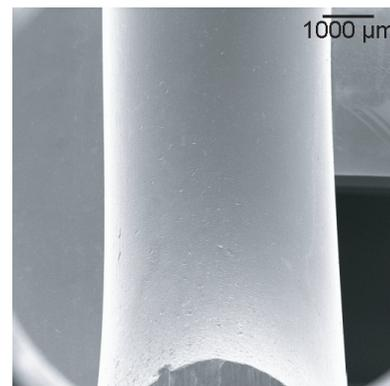
Figure 4: SEM micrograph of PBG iris.
