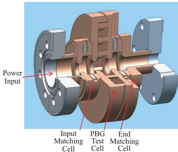
Figure 1: Single cell standing wave PBG structure.
