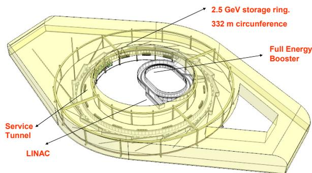
Figure 2: Preliminary general lay-out of the LNLS-2 light source.
