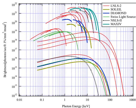
Figure 1: Brightness from various insertion device and bend magnet sources at LNLS-2 (red curves) and from a typical devices in other sources.
