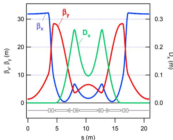
Figure 3: Lattice Functions for the LNLS-2 Light Source.
