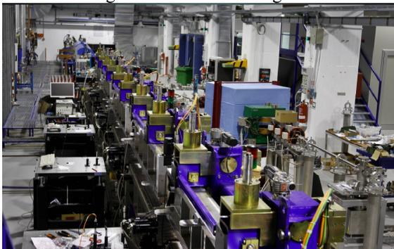
Figure 2: Photo of the SPARC undulator sequence.
