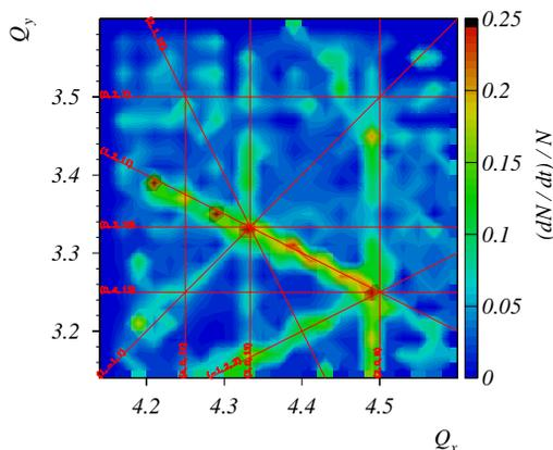
Figure 1: SIS18 measured beam loss as function of tunes.
