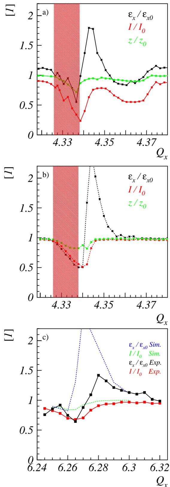
Figure 2: a) Transverse-longitudinal beam response to the long term storage as function of working points around the third order resonance; b) Simulation of picture a). c) Result of CERN-PS measurements, and in dashed lines simulation result on modeling (case where chromaticity is included).
