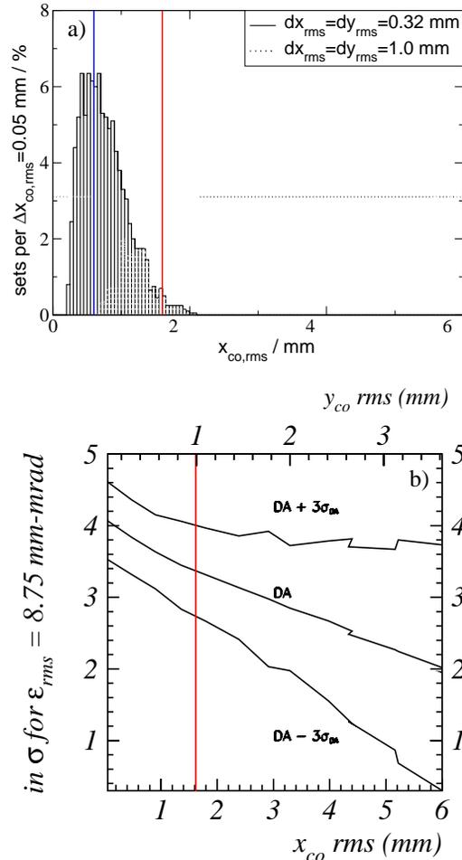
Figure 1: a) Closed orbit distortion after correction for two sets of closed orbit errors: the normal positioning error of 0.32 mm, and for example for the enhanced level of 1 mm; b) DA computed for several error seeds defining an rms COD.
