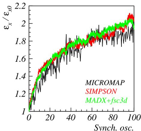
Figure 4: Emittance growth versus synchrotron oscillations in 3 different codes.
