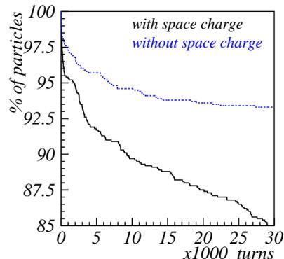
Figure 5: Long term beam loss for SIS100 beam2 including space charge (black) and without (blue).
