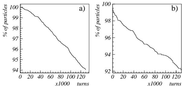
Figure 3: SIS100 beam loss with space charge for Beam1 a) and Beam2 b) for an intensity of  $3 \times 10^{11}$  ions.
