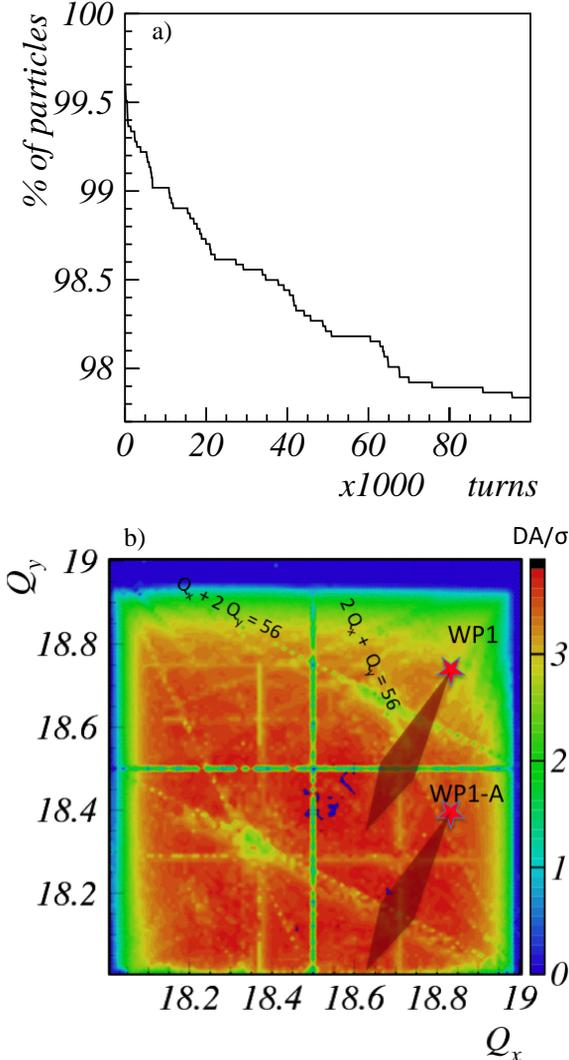
Figure 2: a) Beam2 for the standard error case. b) SIS100 dynamic-aperture scans for the “standard error seed”. Red marker: proposed working point WP1.
