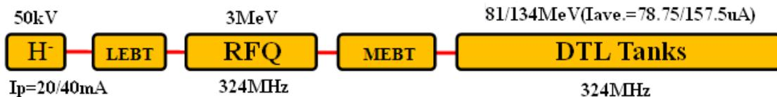
Figure 1: Layout of CSNS Linac.
