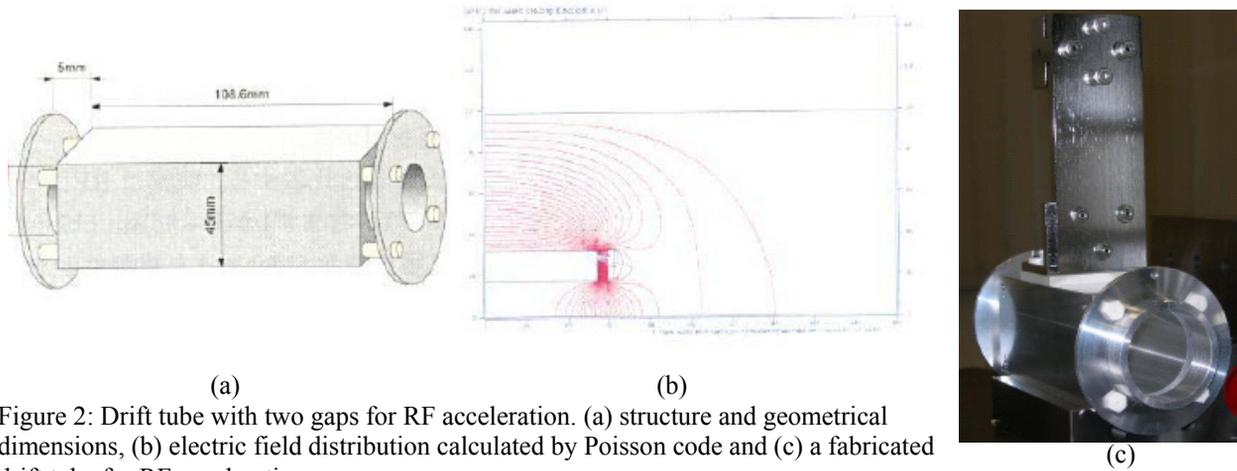
Figure 2: Drift tube with two gaps for RF acceleration. (a) structure and geometrical dimensions, (b) electric field distribution calculated by Poisson code and (c) a fabricated drift tube for RF acceleration.
