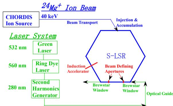
Figure 3: Schematic view of a longitudinal laser cooling system of  $^{24}\text{Mg}^+$  ion beam at S-LSR.
