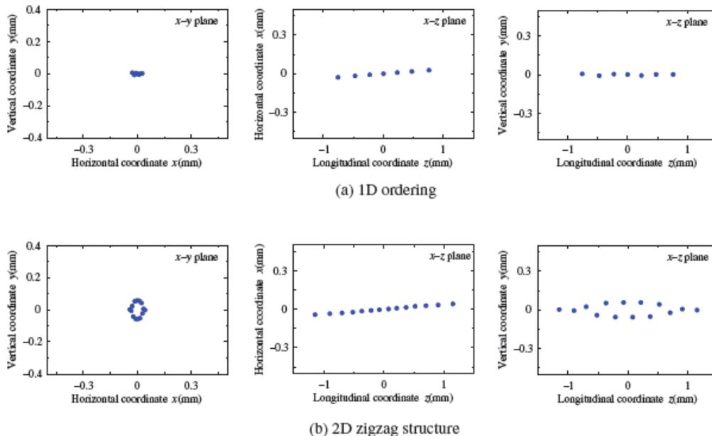
Figure 5: One (a) and two (b) dimensional crystalline beam expected at S-LSR by a MD simulation. (from Ref. [12])
