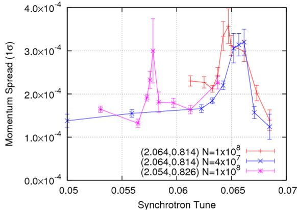
Figure 4: Dependence of the equilibrium momentum spread after bunched beam laser cooling on the synchrotron tune.
