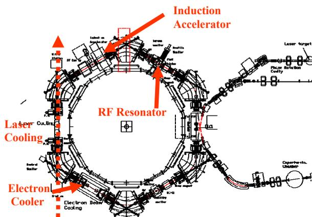
Figure 1: Layout of an ion storage and cooler ring, S-LSR. Laser cooling is applied to  $^{24}\text{Mg}^+$  ion beam at one of 6 straight sections.
